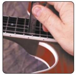
Step 4. Setting Your String Height Players with a light touch can get away with lower action, others need higher action to avoid rattles. Check tuning. Using 6" ruler, measure distance between bottom of strings and top of the 17th fret. Adjust bridge saddles or if your saddles are preset, the bridge height adjustment screws, to approximately 4/64". Experiment with the height until the desired sound and feel is achieved.
